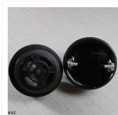
PIEZO ELECTRIC ALARM WITH INTERNAL CIRCUITRY
