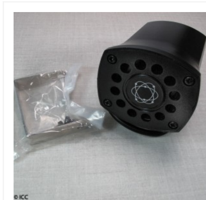
PIEZO HORN WITH BUILT-IN CIRCUIT AND MOUNTING BRACKET
