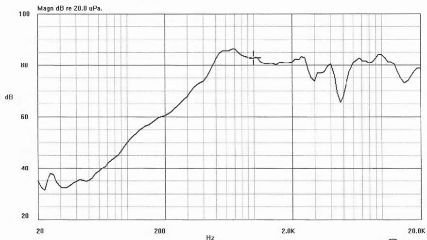
Current Curve: 0 X: 1000 Hz Y: 82.90 dB Time[Y/M/D H:M:S]: 2005/12/ 8 7:17:22
