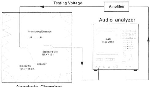
Anechoic Chamber 480\*420\*360 cm Chamber F
