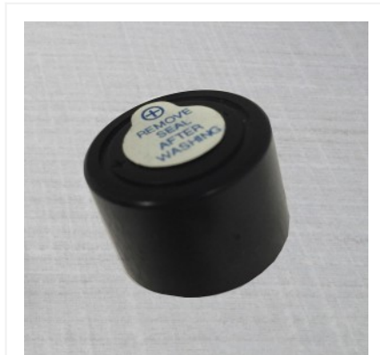
PIEZO ELECTRIC ALARM WITH INTERNAL CIRCUITRY
