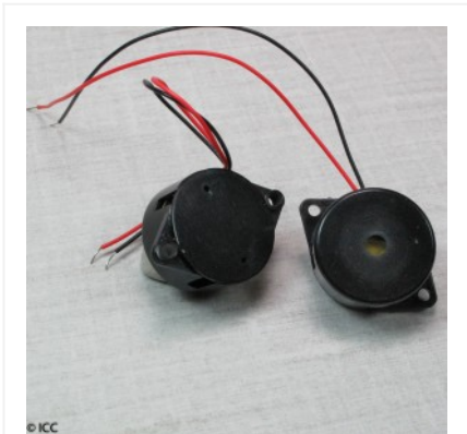
PIEZO ELECTRIC ALARM WITH INTERNAL CIRCUITRY
