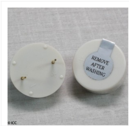
PIEZO ELECTRIC ALARM WITH INTERNAL CIRCUITRY
