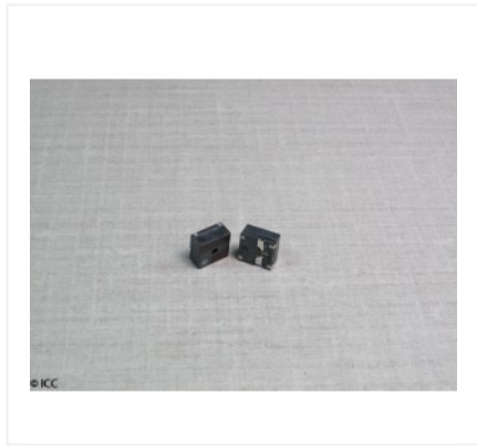
SURFACE MOUNT ELECTRO-ACOUSTIC TRANSDUCER
