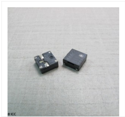
SURFACE MOUNT ELECTRO-ACOUSTIC TRANSDUCER
