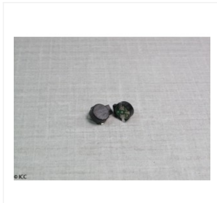
SURFACE MOUNT ELECTRO-ACOUSTIC TRANSDUCER
