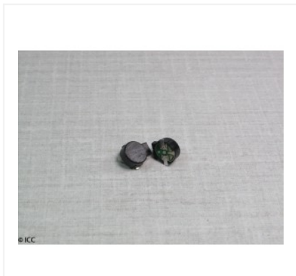
SURFACE MOUNT ELECTRO-ACOUSTIC TRANSDUCER
