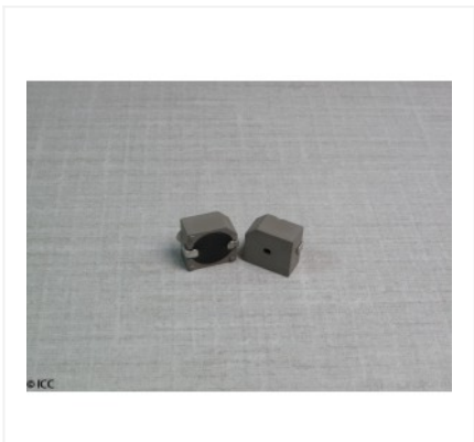
SMT TRANSDUCER WITH BUILT IN CIRCUIT
