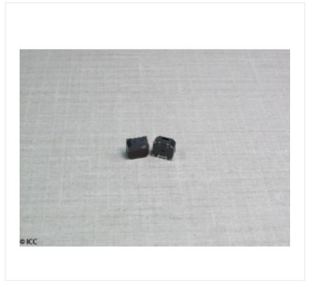
SURFACE MOUNT ELECTRO-ACOUSTIC TRANSDUCER
