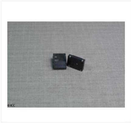
SURFACE MOUNT ELECTRO-ACOUSTIC TRANSDUCER
