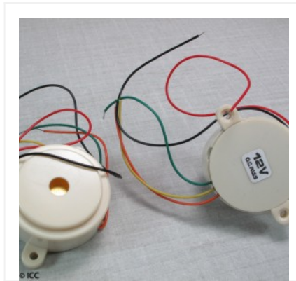
PIEZO SOUNDER WITH BUILT-IN CIRCUIT
