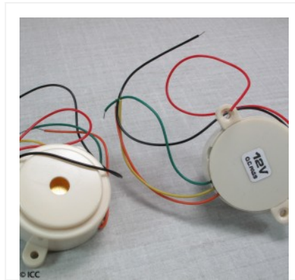
PIEZO SOUNDER WITH BUILT-IN CIRCUIT
